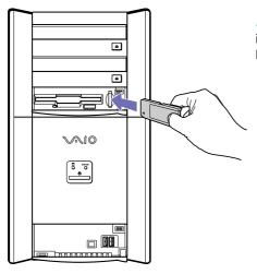
Always hold the Memory Stick<sup>TM</sup> with the arrow pointing in the correct direction when you insert it into the slot. To avoid damaging the computer or the Memory Stick<sup>TM</sup>, do not force the Memory Stick<sup>TM</sup> into the slot if it does not insert smoothly.
